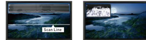
Displays the waveform for a signal that is input at any desired line (shown by the white line).
